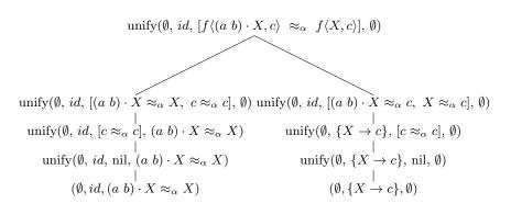
Example 6. Suppose f and g are commutative function symbols, and h is a non-commutative function symbol. This example shows how the algorithm would unify  $g\langle h \ d, f\langle (a \ b) \cdot X, c \rangle \rangle$  with  $g\langle f\langle X, c \rangle, h \ d \rangle$ . Because g is commutative, the algorithm explores two branches:
